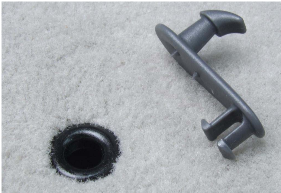
Figure 4 –Floor Mat Retaining Clip and Carpet Receiving Eyelet
