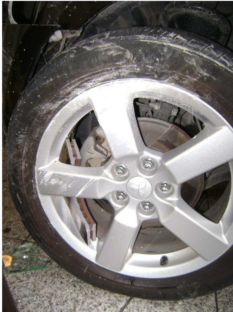
From Fig 10: Broken off segment of LH front Disc Brake Rotor
