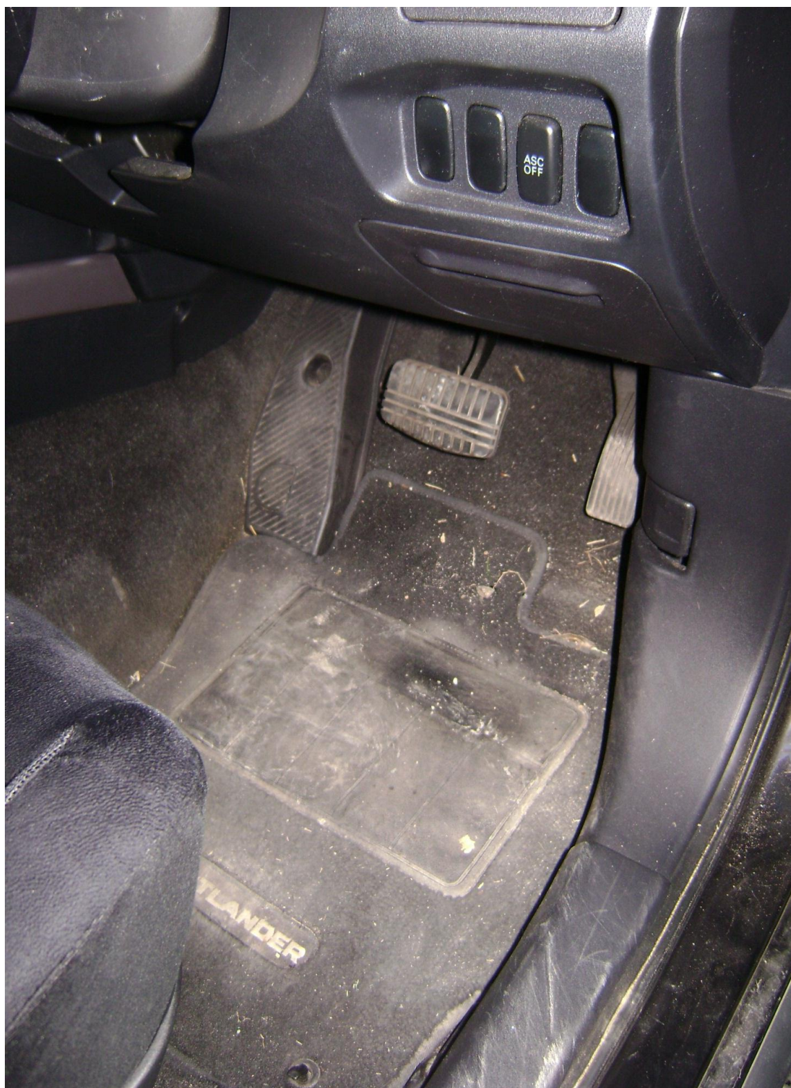
Fig 16 Brake and Accelerator pedal arrangement. Most of the heel wear on the floor mat seems more or less in the middle of the mat. (Police photograph)
