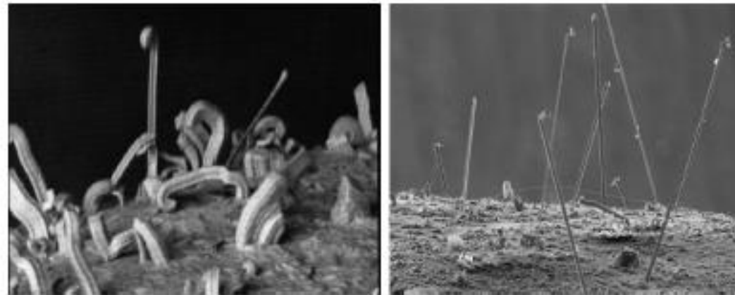
FIG. 1. Scanning electron microscope (SEM) pictures of tin (left) and zinc (right) whiskers. Courtesy of the NASA Electronic Parts and Packaging (NEPP) Program [6].
